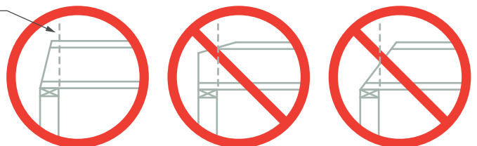
Diagram D16: skewed joist support fixing
